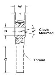
**Body:** Carbon steel, protective coated for corrosion resistance.
